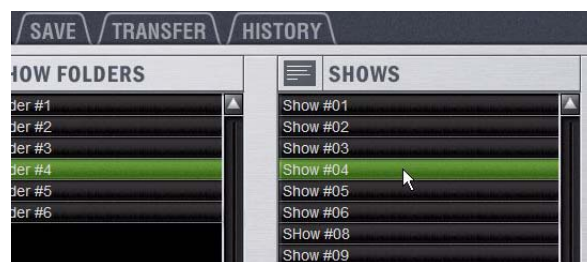
Show Folders and Show files in the Load tab of the Filing Page
