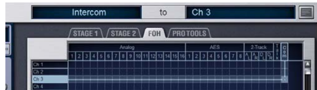
Routing Intercom input in the Patchbay
