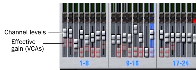
Effective gain (VCA contribution) shown in the on-screen fader displays
