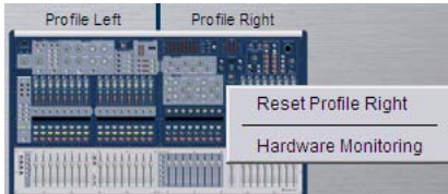
Resetting a unit in the Options > Devices page
