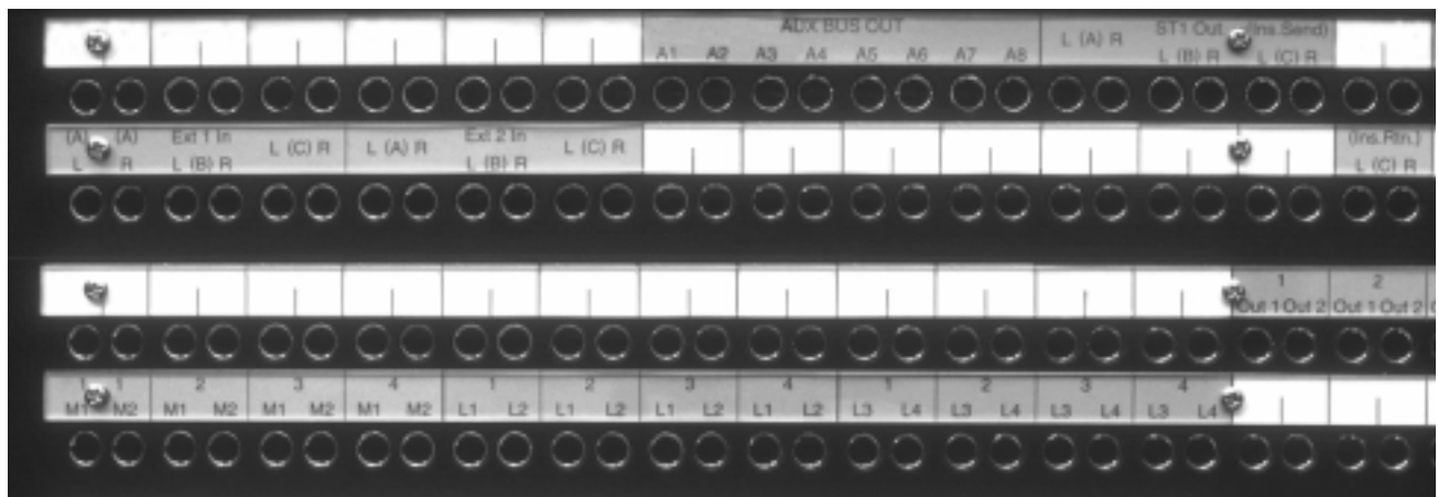
Front of patchbay showing Master patch unit and Channel patch unit.
