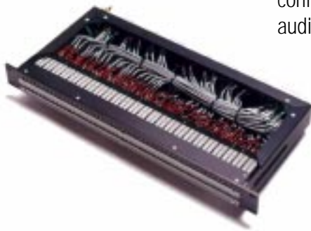
Euphonix Patchbay. There are two 48-jack rows of half-normalled TT jacks on the front, and Elco connectors on the rear panel.
