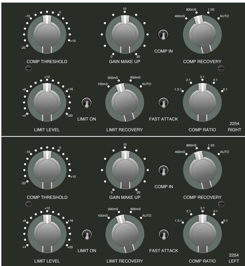
The control characteristic is shaped such that the onset of compression is smooth and progressive, the true ratio being reached within the first 5 to 10dB above the Threshold.
